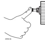
now disarm. If the system does not disarm, you may have waited too long to press the Valet® switch; turn the ignition off and repeat the process.
